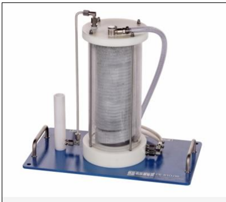
Figura 18. Reactor PFR Helicoidal
