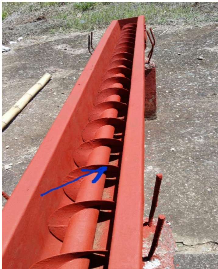
Figura 7. Aspas del conductor helicoidal
