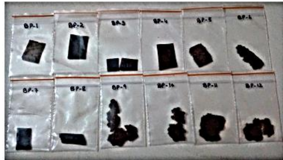
Fig. 1. Showing the twelve different banana peel starch based bioplastic samples produced.
