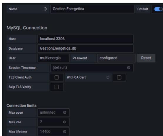
The image shows the Grafana configuration interface for a MySQL connection. At the top, the connection is named "Gestion Energetica" and is set to "Default". The "MySQL Connection" section includes the following fields and options:
