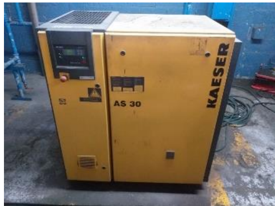
Figura 16. Compresor Kaeser AS 30 – 30 HP
