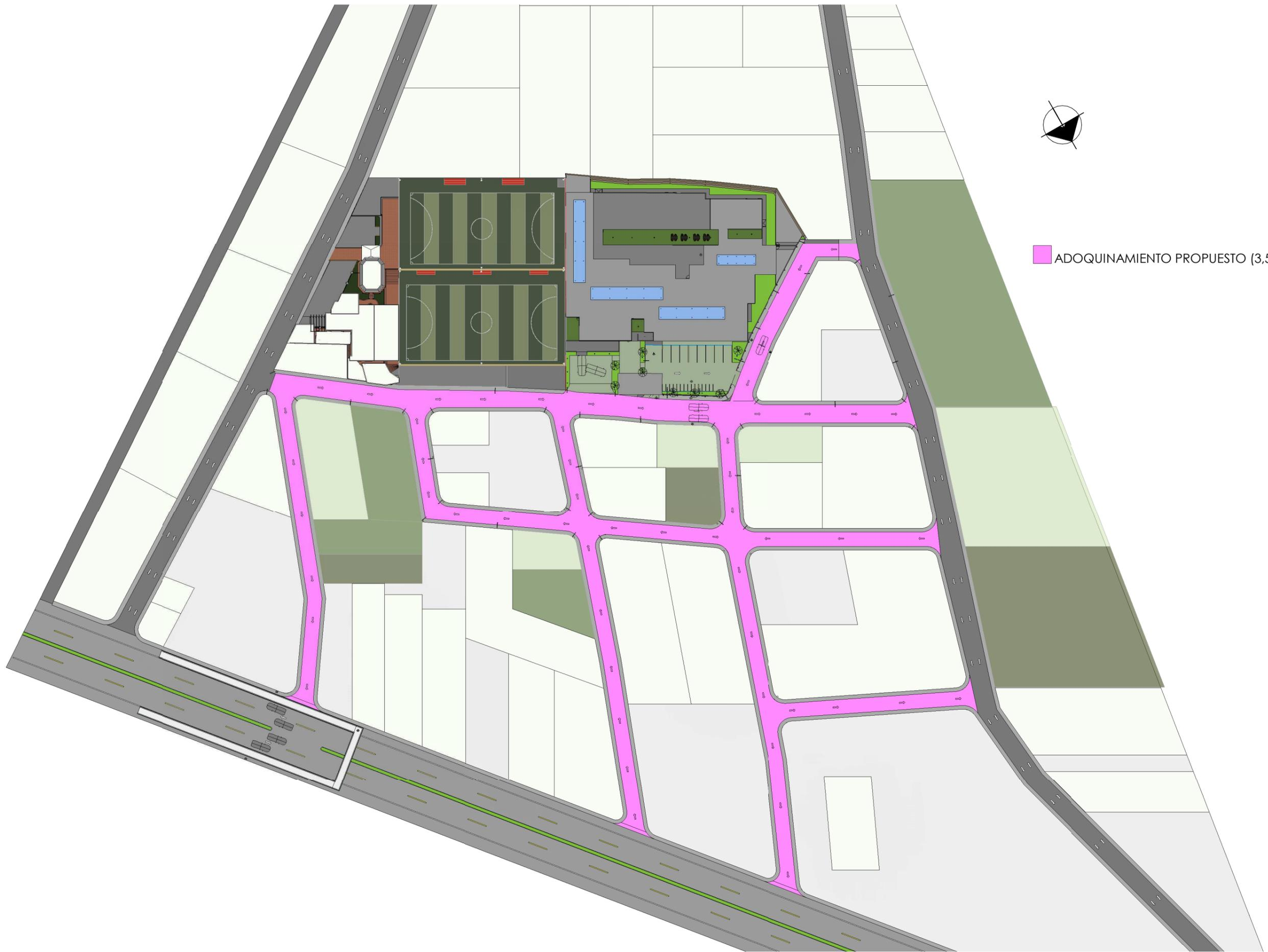
ADOQUINAMIENTO PROPUESTO (3,541 m<sup>2</sup>)
