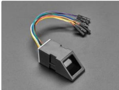
If your fingerprint sensor has individual socket wires (its this one) (<https://adafru.it/QfT>) then use the following wire setup:
