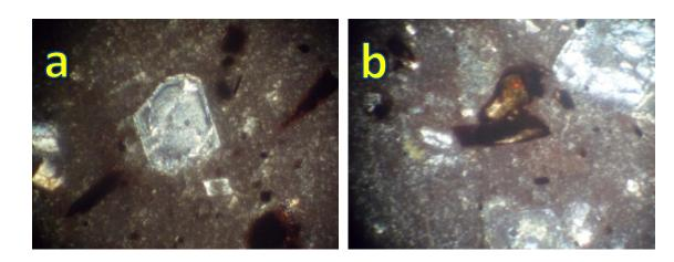
FOTOGRAFÍA HORNBLENDA ALTERADA DISTINGUIÉNDOSE SU FORMA TABULAR, FELDESPATOS PPL
