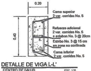
**DETALLE DE VIGA L-L'**
