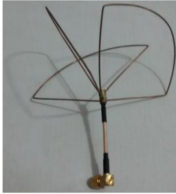
Fuente: *1.2 GHz Circular Polarized Antenna SMA (Set) (Short)*.
